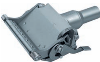
GB231R GB682R micro-Line Dermatome acc. to Wagner cutting width keyless adjustable; thickness adjustable (1/10 mm steps); cutting thickness: 0.2 - 1.2 mm; cutting width: max. 78 mm 6:1; \updownarrow 3.0 mm; \updownarrow 770 g consisting parts: GB228R blades
